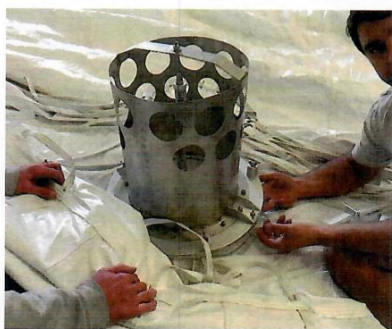
Above: Fitting the stainless steel valve that sits at the top of the balloon in the middle of the crown ring, opening automatically as the balloon ascends.
