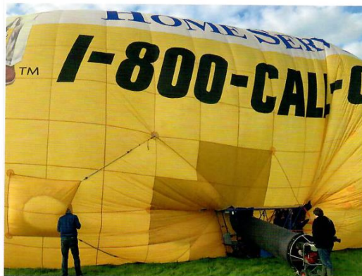
Above: The envelope is cold-inflated via a tube attached to the fan.
